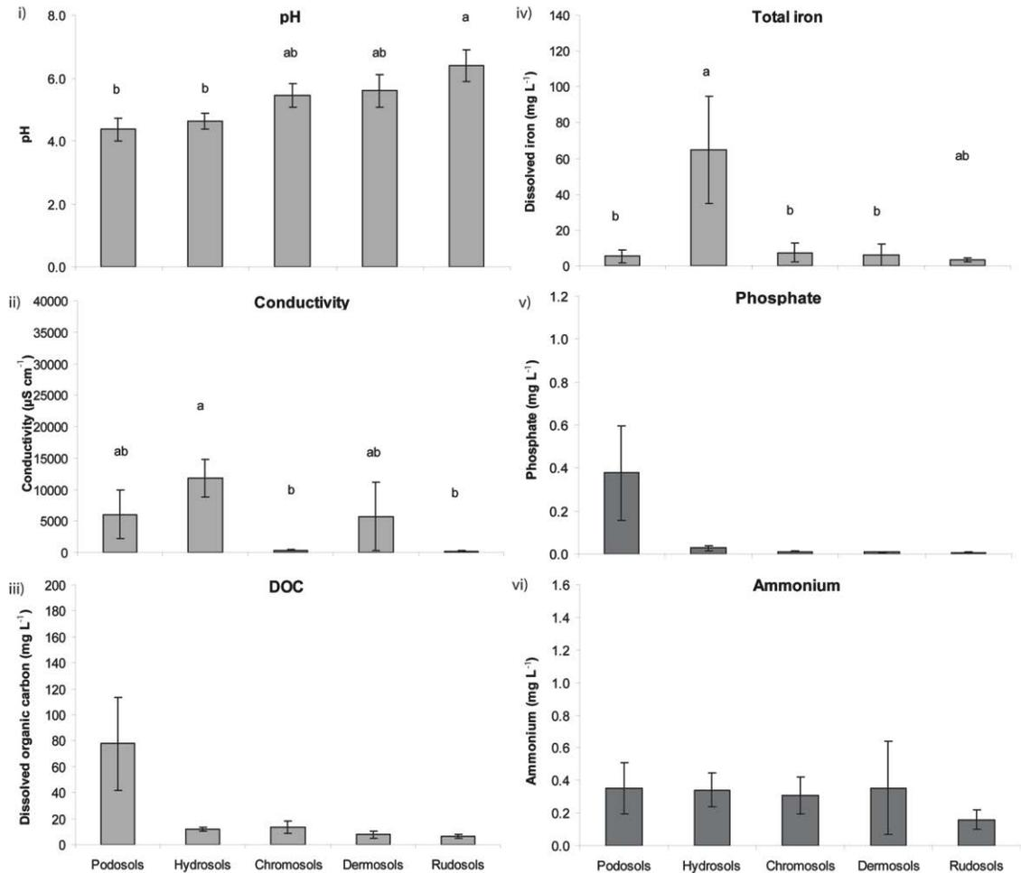
FIG. 4. Mean ( $\pm$ SE) of nutrient concentrations and properties of the groundwaters collected from different soil orders in the Deception Bay/Bribie Island study area: (i) pH; (ii) conductivity; (iii) DOC; (iv) total iron; (v) total phosphorus; and (vi) ammonium. Means followed by a common letter are not significantly different at  $P > 0.05$ . ANOVA for DOC and ammonium were not significant ( $P > 0.05$ ).
